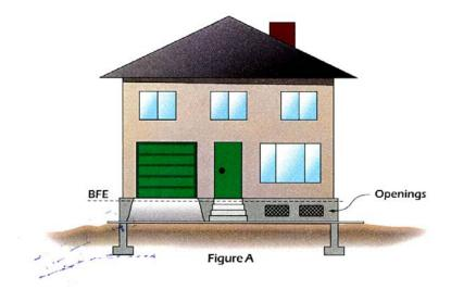
The illustration below shows a standard crawlspace design that is NFIP compliant and not expensive to insure. Note that the interior grade and exterior grade are the same, vents are properly shown no higher than one foot above grade and all ductwork and utilities are located above BFE. If the flood vents were not present in the illustration below, the lowest floor would be the elevation of the interior grade as shown, well below BFE and much more expensive to insure.
