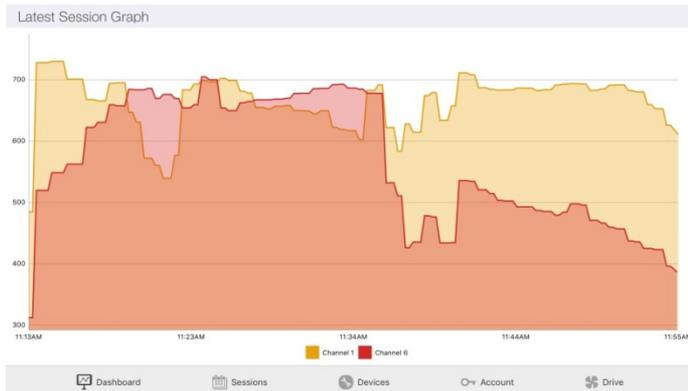
AFTER 25 MINUTES THE DRY WOOD BURN IS HOLDING AT 610 DEGREES, WHILE THE WET WOOD BURN IS DOWN TO 384 DEGREES.
