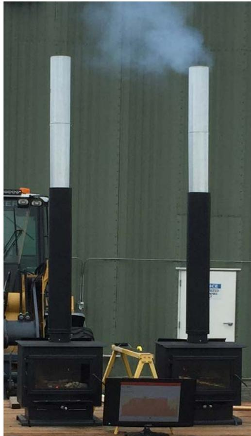
WITHIN 6 MINUTES, THE STOVE WITH DRY WOOD HAS NO VISIBLE SMOKE AND STOVE TEMP IS 700 DEGREES. THE STOVE WITH WET WOOD IS SMOKING AWAY, AND STOVE TEMP HAS DROPPED TO 530 DEGREES.
